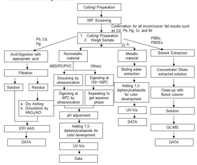
Note: 1) Boiling water test method was also performed for Cr (VI) analysis in metal sample.
